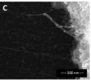
Nanostructuring is clearly observed with nanotubes. IrOx forms around them in layers, while the nanotube supports the oxide structure as a scaffold. The final material es among the most supporting of neural cell growth.
